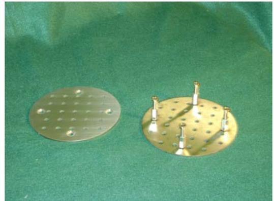
Six inch round stainless steel Talk Thru has offset holes in front and rear to allow natural voice transmission. Talk Thru is available as interior or exterior model (specify). It fits glass from 1/4" inch to 1 7/8 " thick. Denote glass thickness of window when ordering Talk Thru.
