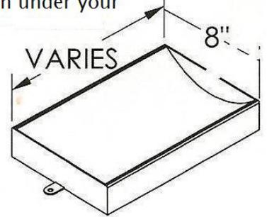
**CXCM D&C** Stainless steel counter top model deal tray mounts on top of counter. No cut out is required. Secured with screws through countersunk holes into your existing risers.
