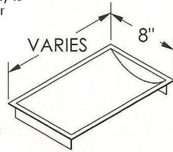
**CXR (WITH BULLET TRAP)** For added security, add optional bullet trap to any stainless steel trays.
