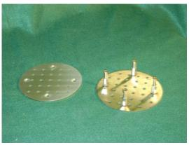
Six inch round stainless steel Talk Thru has offset holes in front and rear to allow natural voice transmission. Talk Thru is available as interior or exterior model (specify). It fits glass from 1/4" inch to 1 7/8 " thick.
