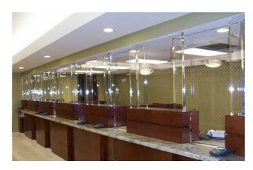
Plastic laminate with integrated Bullet Resistant Barrier.
